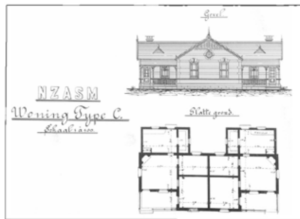
Figure 2 Plan and elevation of Type C: Semi-detached cottage (NZASM drawing) (De Jong, Van der Waal and Heydendrych 1988).
