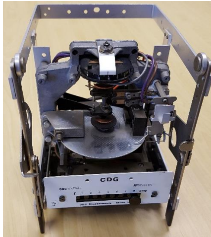
Figure 4.8. An induction disk electromechanical protection relay.
