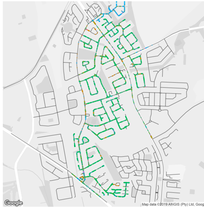
Figure 4.11: GPS points grouped by vehicle ID for the service area
