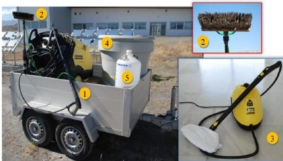
Figure 2.14. Pressure washing device with hand spray nozzle accessory (1), water-fed natural horse-hair bristle brush accessory (2), steam cleaner (3), demineralized water tank (4), and additives tank (5). (Source: Raza, et al., 2016)
