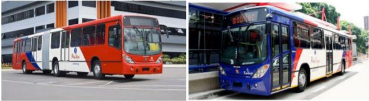
Figure 4:13 Articulated trunk bus and standard feeder or complementary bus in the Rea Vaya system
