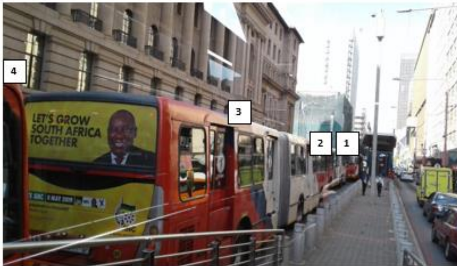
Figure 5:7 Bus bunching at the Library Gardens Station
