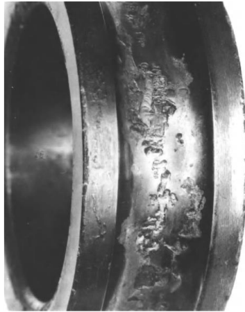
Figure 2.15: Subsurface fatigue wear occurring on a 52100-ball bearing race (Bhushan, 2013: 344).
