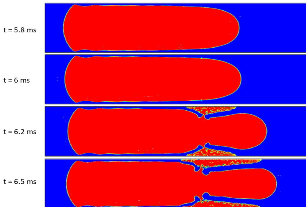
Figure 3-4: Vapour slug profile (red) as it enters the heated region from 5.8 to 6.5 ms without smearing the mass transfer
