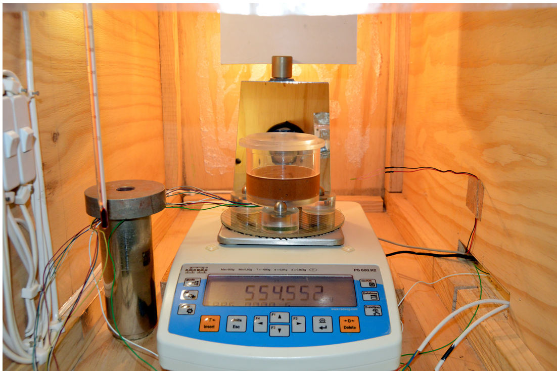
Figure 4-12 Continuous drying test set-up in the enclosure
