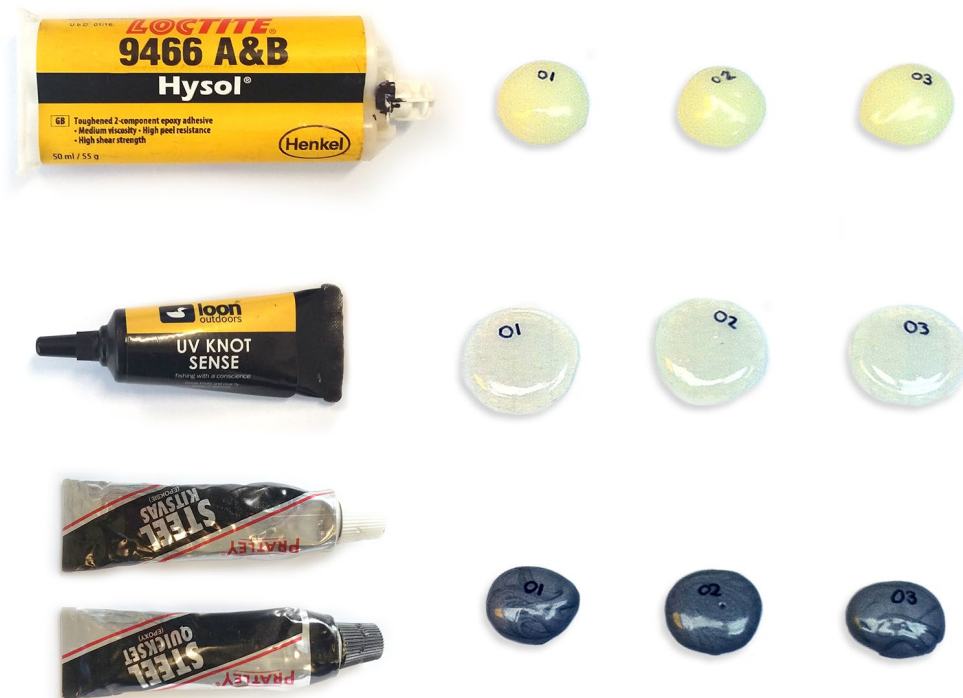
Figure 3-6 Structural epoxy samples for water absorption test
