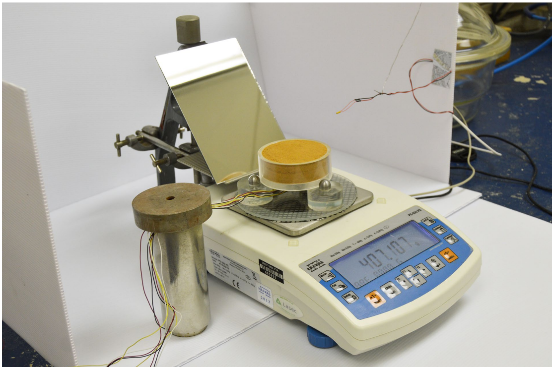
Figure 4-8 Continuous drying test set-up during testing
