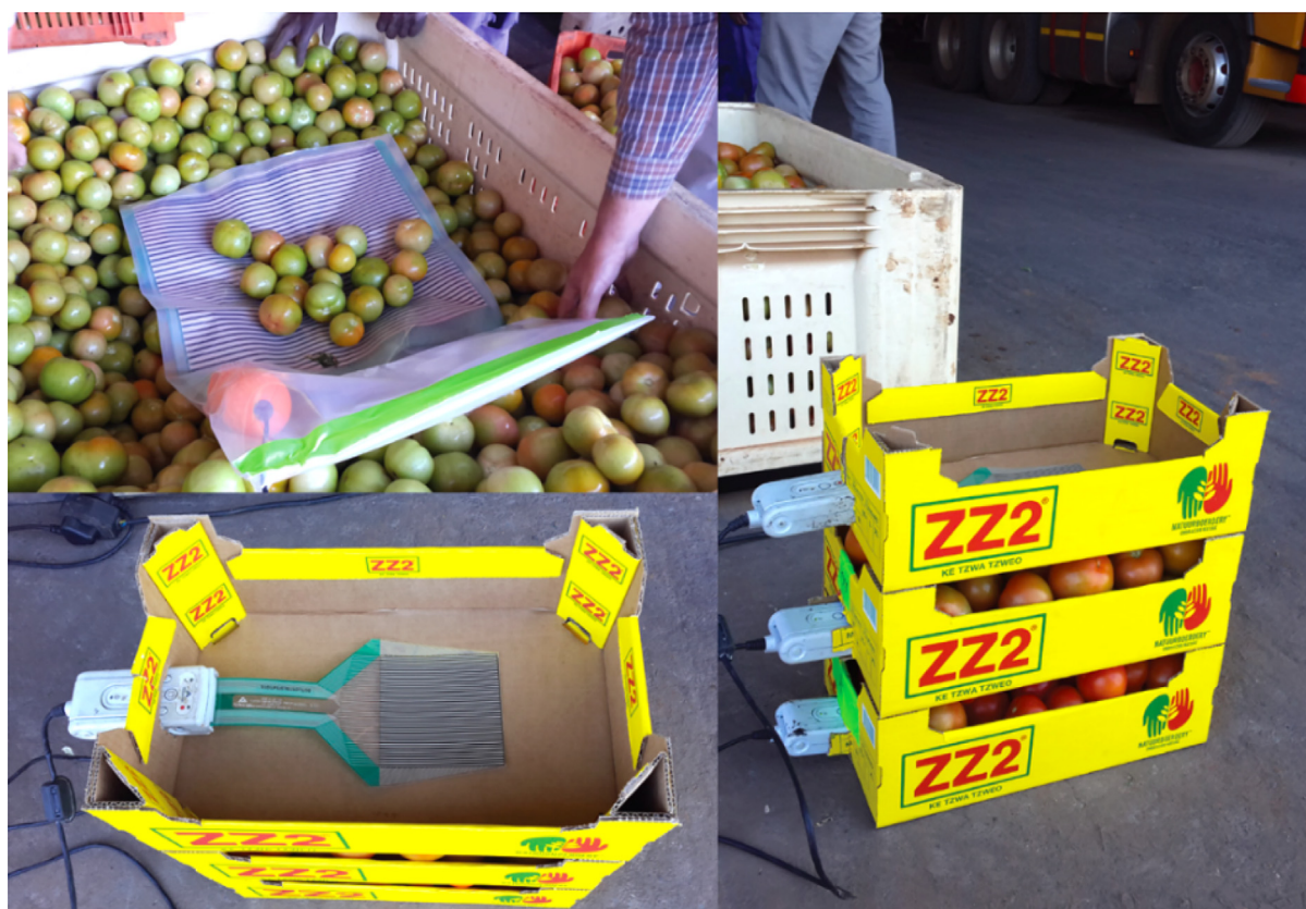
Fig. 1. Pressure sensor matrix for measuring interfacial tomato stresses during transit (from [11]).
