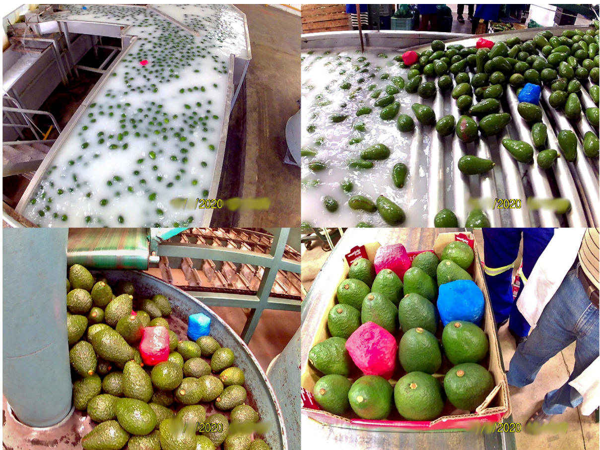
Fig. 15. Avocado packhouse illustrating the postharvest treatment (top-left), drying (top-right), sorting (bottom-left) and packing (bottom-right) processes.
