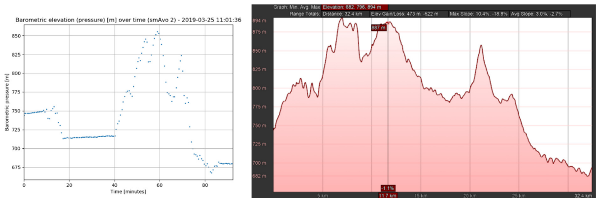
Fig. 14. Comparison between the measured barometric air pressure measured by smAvo (left) and an elevation profile obtained from Google for the same route (right).
