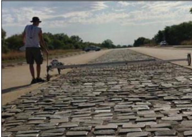
Figure 16: Belgian paving track at Gerotek (Hamersma & Els, 2014)
