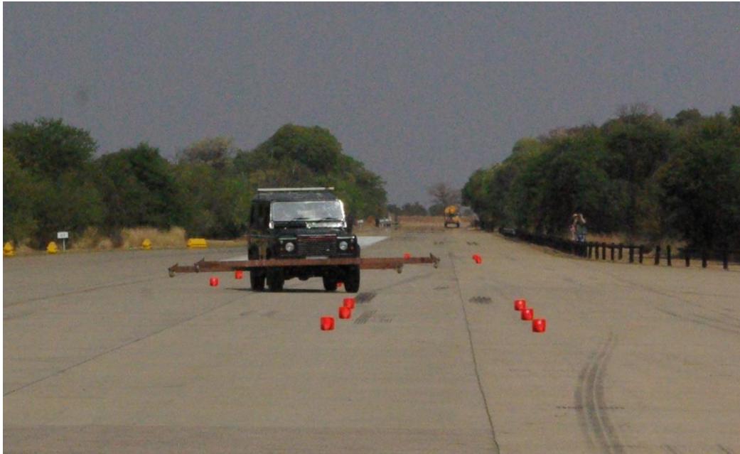
Figure 14: Land Rover performing a double lane change manoeuvre at Gerotek
