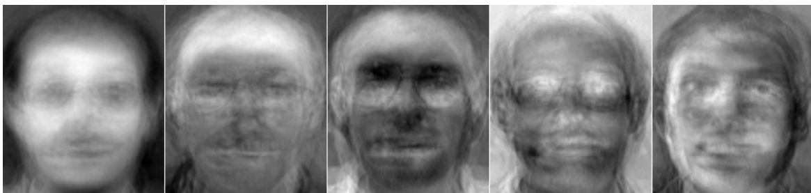
Figure 3.4. From the left, the average face and the first 4 eigenfaces of a set of faces from the AT&T Faces database
