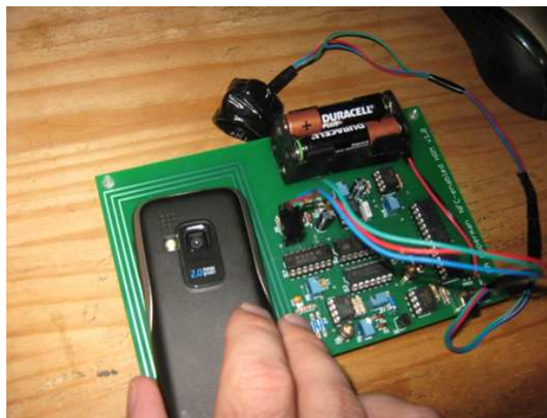
Figure 2.4. A proof-of-concept NFC-enabled heart rate monitor showing how external sensors may be fitted with NFC interfaces to enable communication with mobile devices
