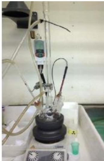
Figure 3-1 Experimental set up for the dissolution of U_3O_8 to prepare a U stock solution
