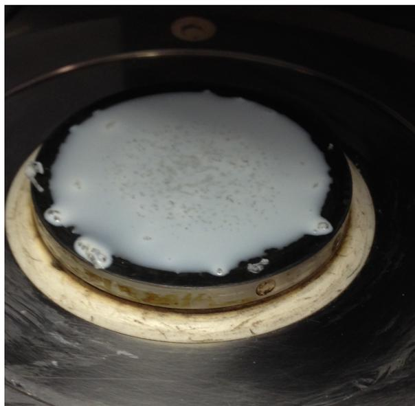
**Figure 3.8:** Photograph of poly(VDF-*co*-HFP) copolymer latex after rheology tests
