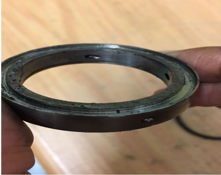
Figure 5.1: Four-hole swirl ring
