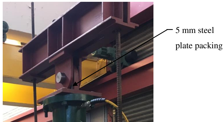
Figure 4-3 Top beam connection stiffening of the press frame
