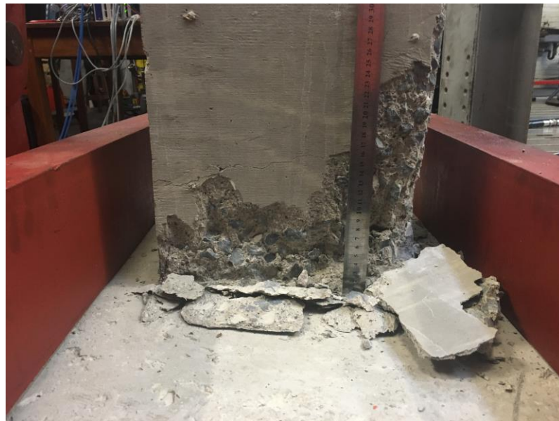
Figure 4-36 Concrete crushing during the 2 g experiment
