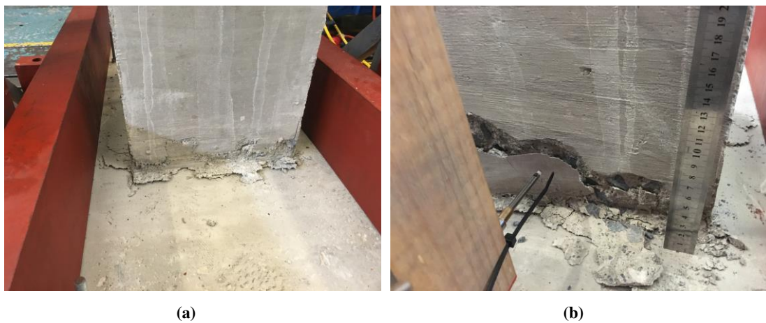
Figure 4-30 Damage and cracking to the footing during the 1 g experiment
