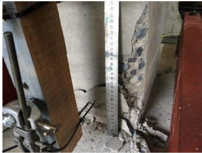
Figure 4-20 Crushing of the concrete after the maximum acceleration had been applied to the footing during the El Centro earthquake at 0.68 g
