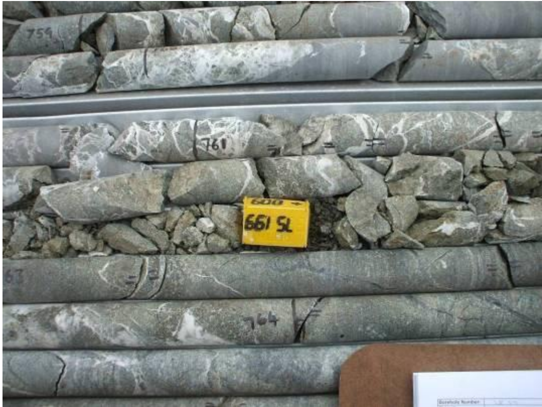
Figure 48: WF59 fault affected area.
