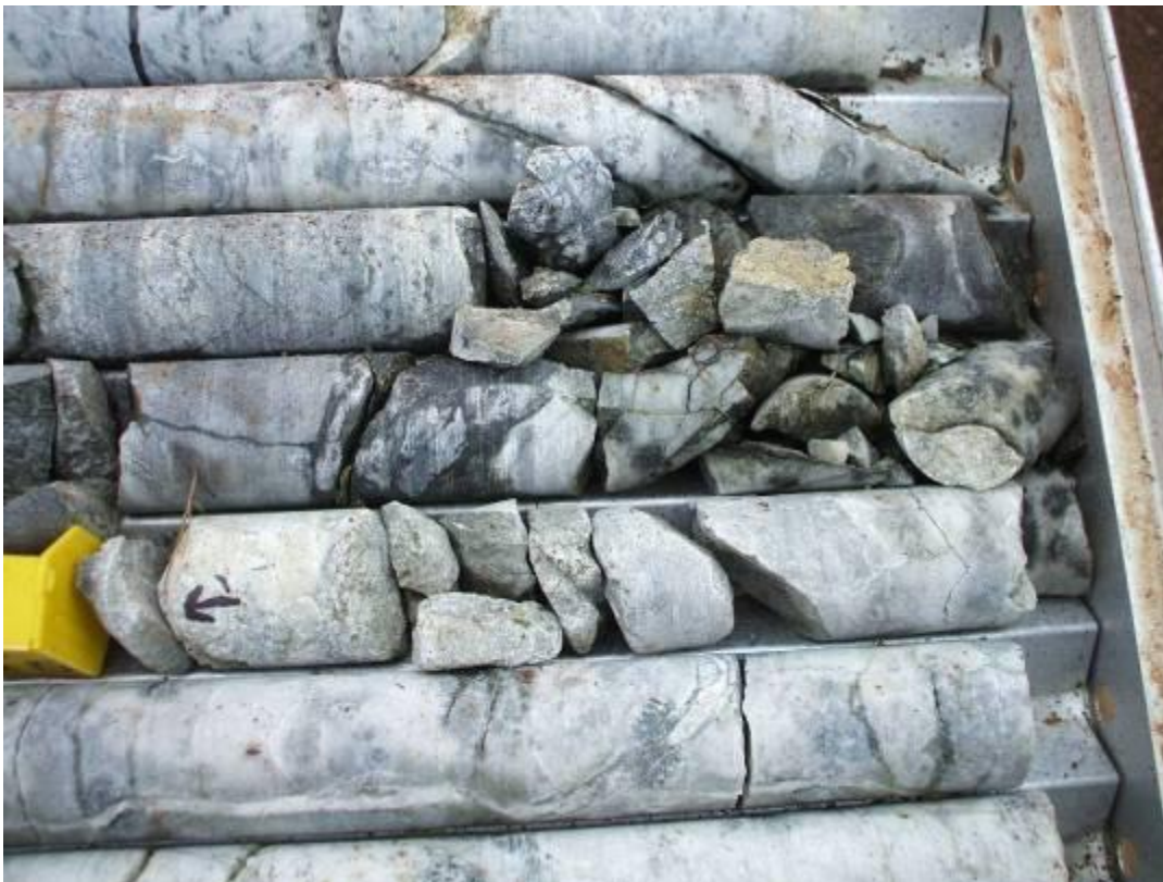
Figure 45: WF49 fault affected area.
