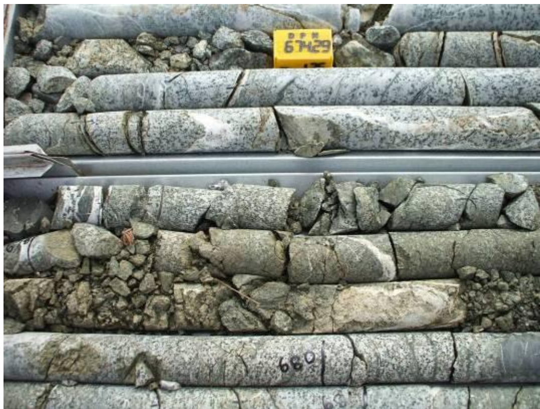
Figure 49: WF90 fault affected area.
