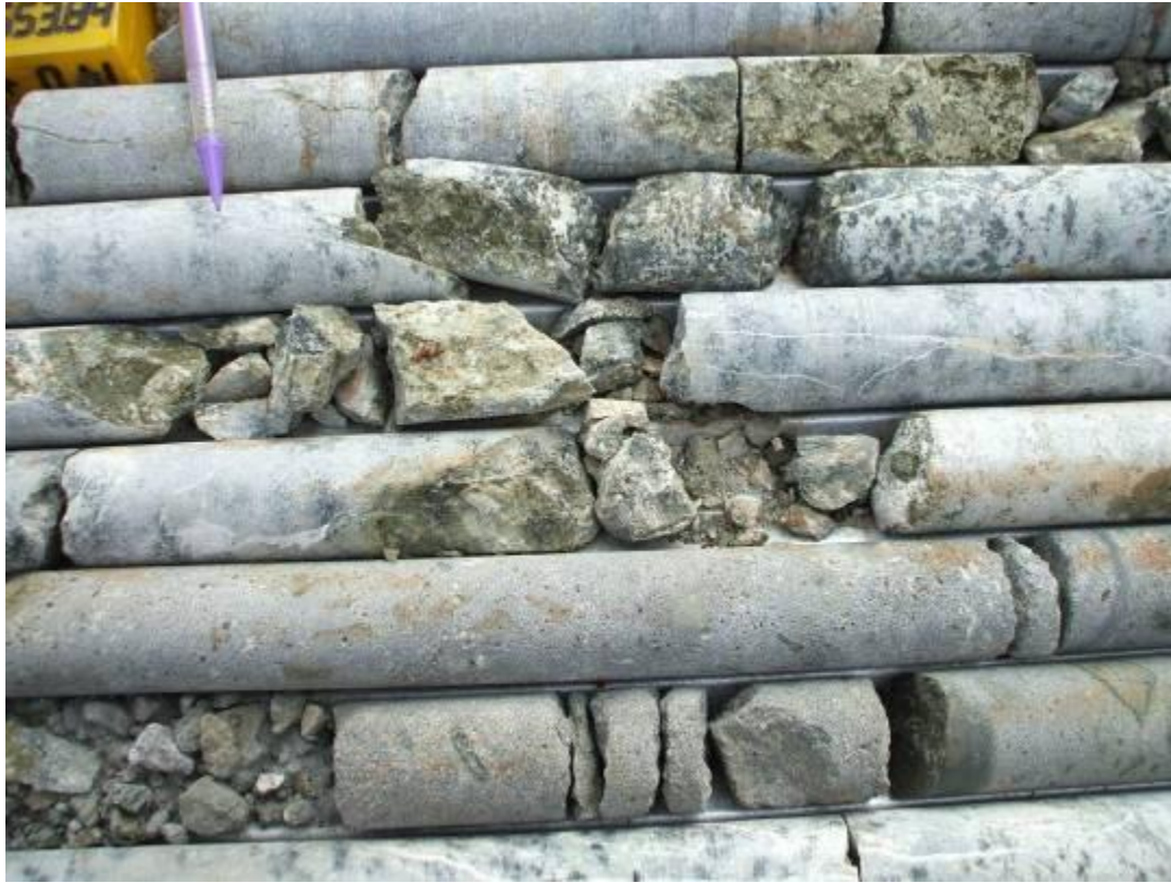
Figure 50: WF90 fault affected area.
