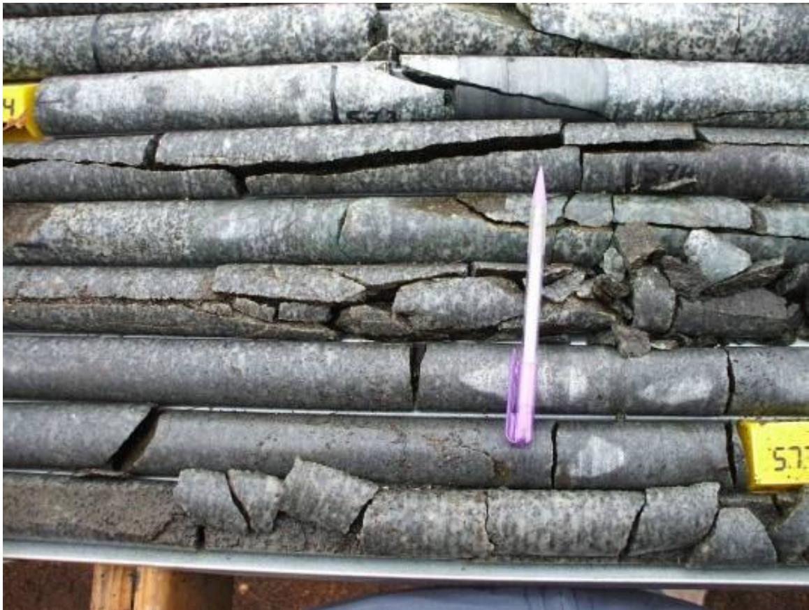
Figure 26: WF1 fault affected area.
