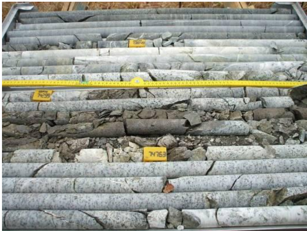
Figure 47: WF59 fault affected area.
