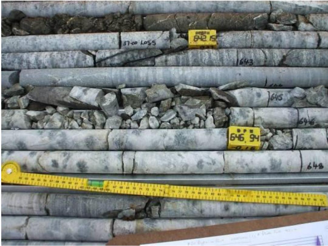
Figure 44: WF49 fault affected area.
