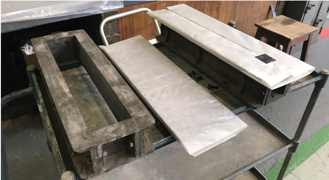
Figure 3.18 Moulds in the process of being wrapped in plastic sample bags filled with baby powder
