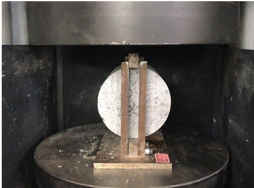
Figure 3.21 Cylinder splitting strength testing setup before being loaded
