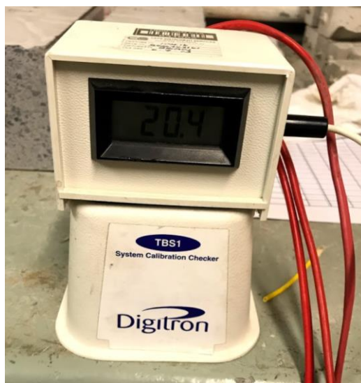
Figure 3.6 Digitron System Calibration Checker used to calibrate thermocouples
