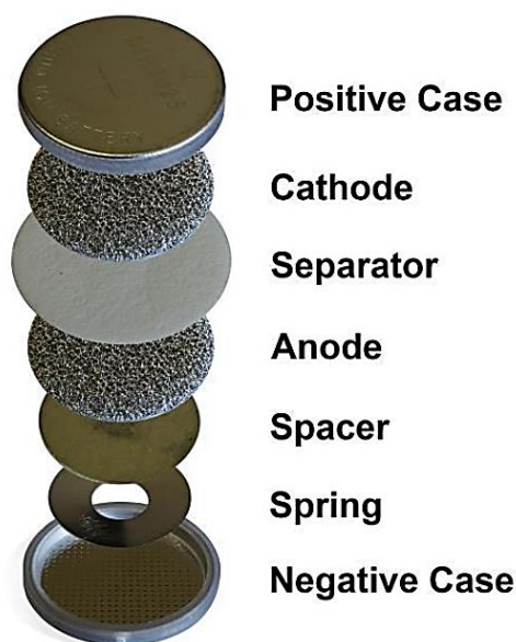
Figure 3.12. Schematic illustration of the assembled structure of supercapacitor device.
