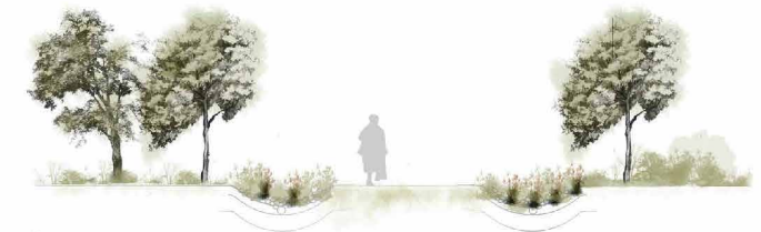
2 Main Catchment: Bio-Swale
