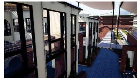
Figure 124: Clear Modek roof sheets on buildings beneath the main pvc roof membrane to let light into the spaces (Author, 2020).
