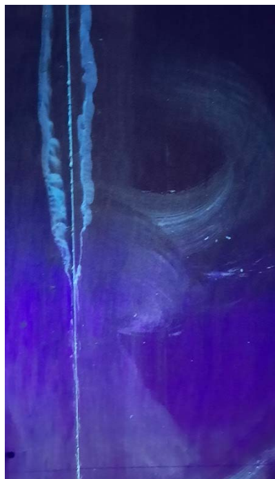
Figure 10: The joint where fluorescence is seen with UV radiation, and the smear made by a piece of cloth or fabric.
