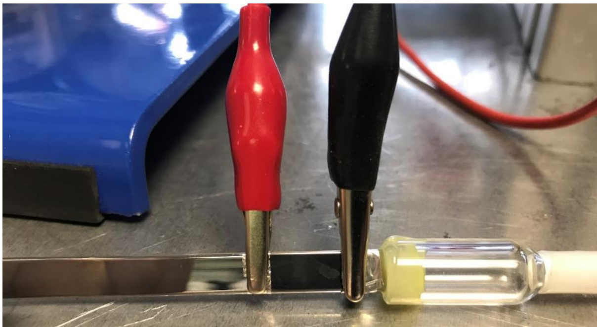
Figure 5: Crocodile clamps attached to the channel to measure its resistance
