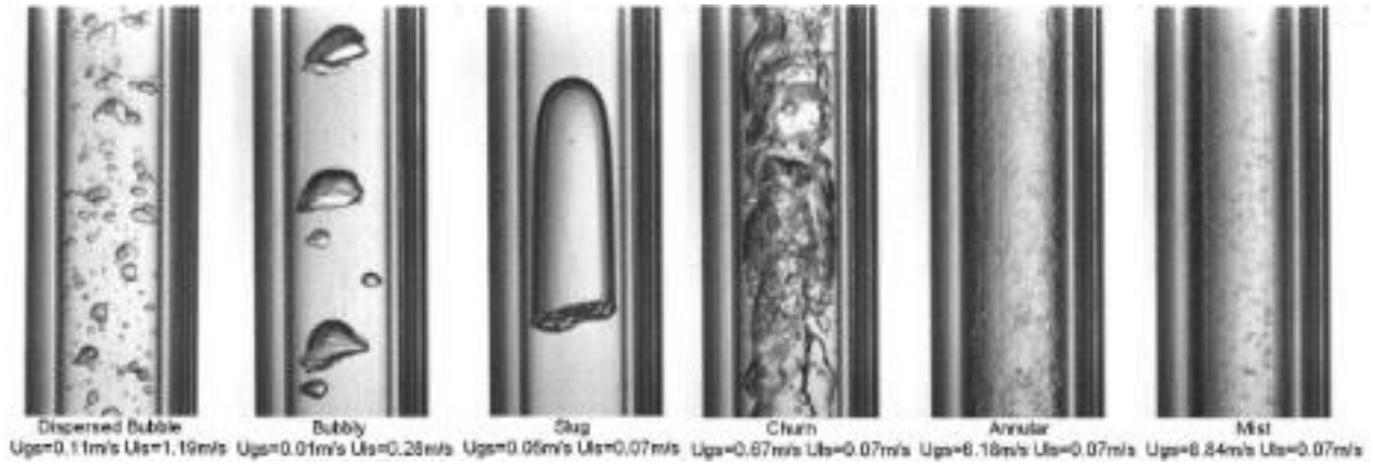
Figure A-8: Flow patterns during upward vertical flow in a 4.26 mm internal diameter tube, taken from Chen et al. [19]
