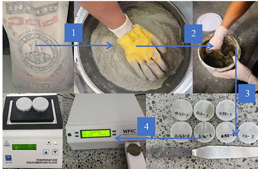
Figure 3-4: Sample preparation steps before suction measurements.
