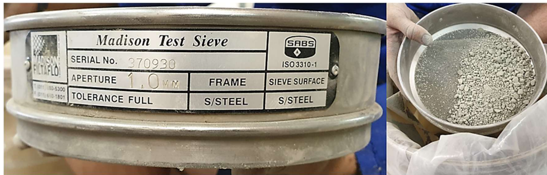
Figure 3-17: Size sieve used to sieve the cement before mixing.
