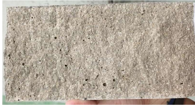
Figure 3-38: Fracture of the split cylinder test sample.
