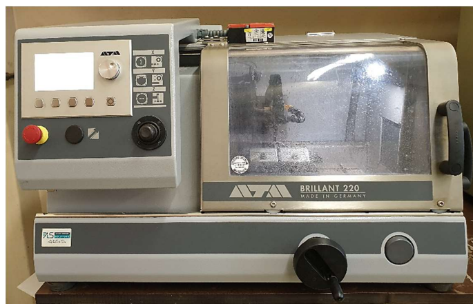
Figure 3-24: Diamond cutting machine used to cut samples.
