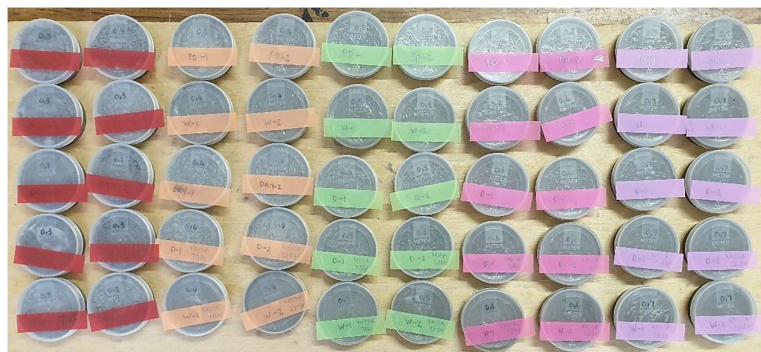
Figure 3-22: Suction samples and porosity analysis samples.
