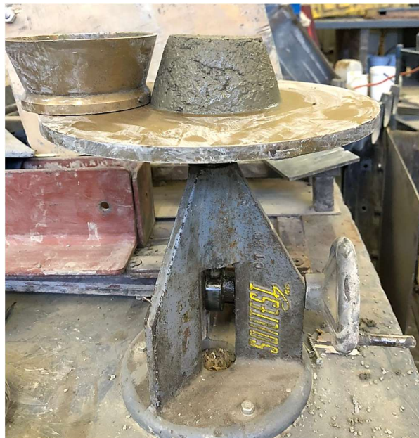
Figure 3-20: Flow table test setup.
