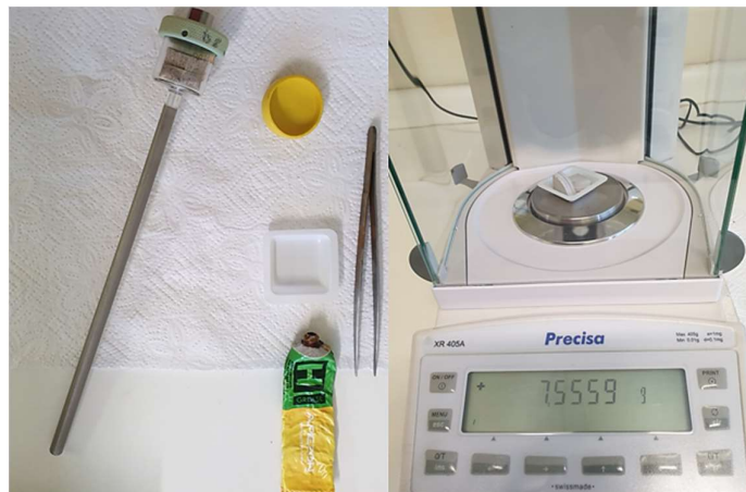
Figure 3-26: Tools required for the sample assembly.
