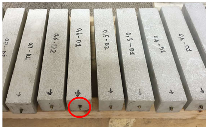
Figure 3-33: Shrinkage beams with anvils on each side.
