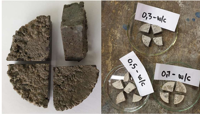
Figure 3-25: Samples sliced in four to be used in the MIP test.
