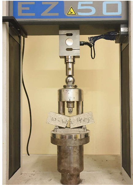
Figure 3-35: Sample failure under TPBT.
