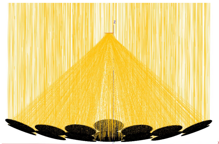
Figure D.6: Traced rays shown in the final numerical solution for the 0 mrad case
