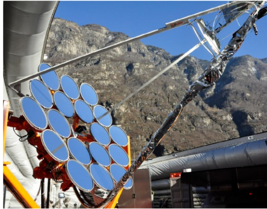
Figure 2-6: Vacuum facet prototype installed in Biasca (Switzerland) during testing (Schmitz et al., 2017)
