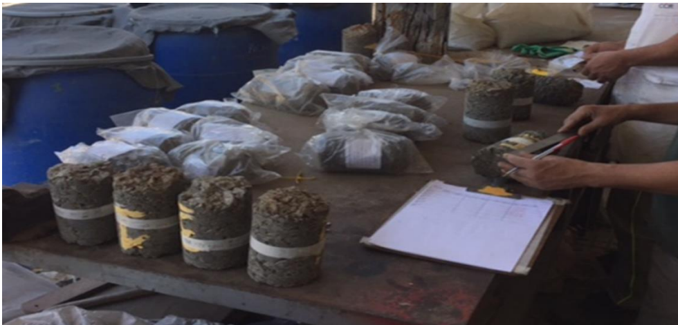
Figure 3-20: Preparation of cylindrical specimens collected from both test sections
