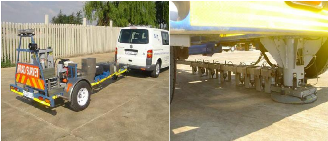
Figure 3-5: FWD Equipment (SANRAL, 2014)
