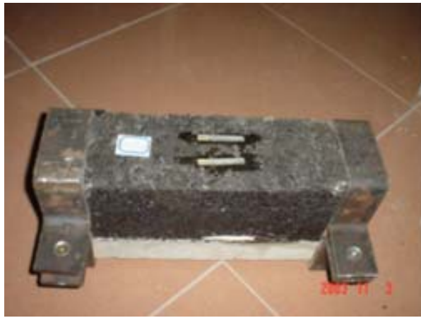
Figure 4. Example of a compound beam sample.
