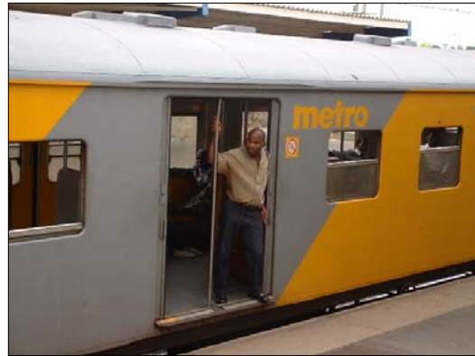
Figure 2. The gap between the platform and train prevents “level access”.
