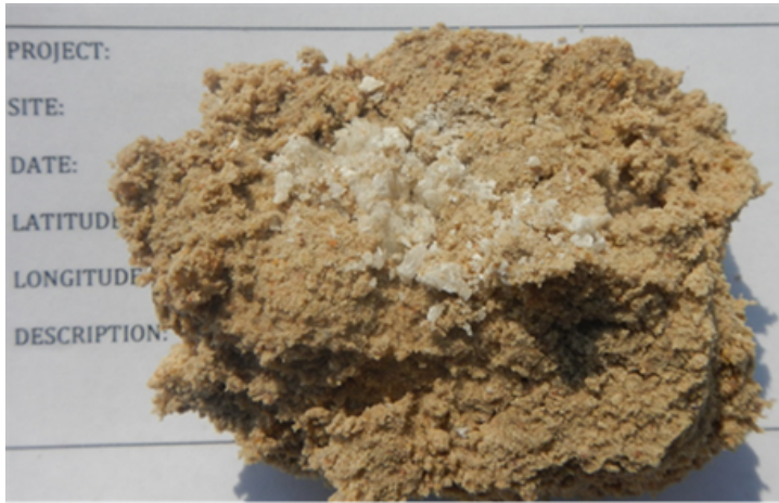
Figure 36: A soil lump with white gypsum precipitate (approximately 5 cm across).
