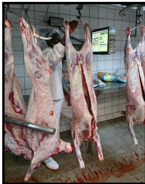
Figure 3.3 Photographic image of the lamb carcass grading system, using Meat Matrix Grading at the Cavalier abattoir
