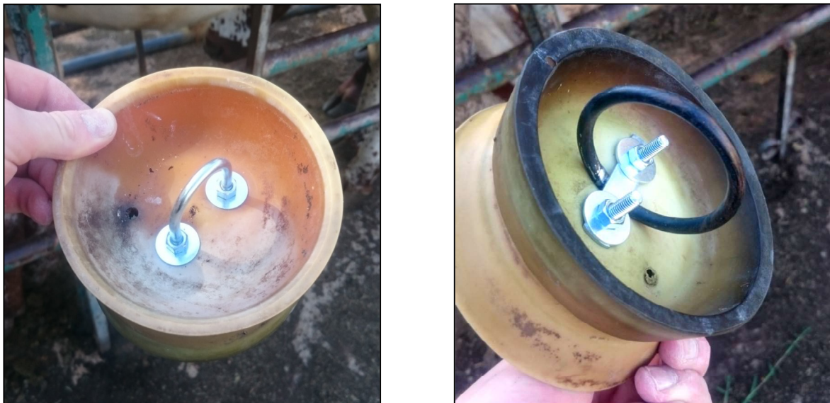
Figure 2: Rumen cannula plug used during experimental trial illustrating the ring used to anchor the in sacco incubation bags in the rumen during the in sacco study of dry matter and NDF disappearance.
