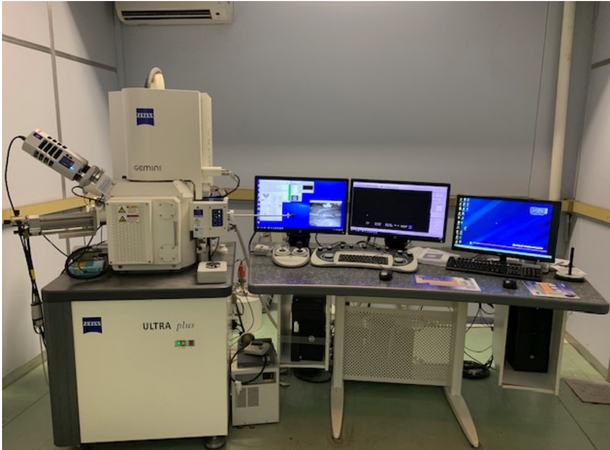
Figure 3.16: High-resolution field emission scanning electron microscope (SEM-Zeiss Ultra Plus 55).
