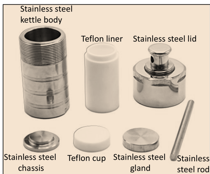
Figure 3.4: Schematic design of a Teflon-lined stainless-steel autoclave.
