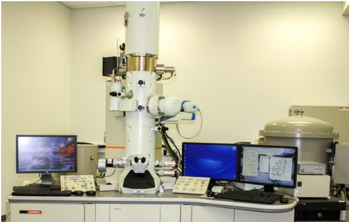
Figure 3.17: High-resolution transmission electron microscope (HRTEM FEI Tecnai-F30 JEOL 2100F).
