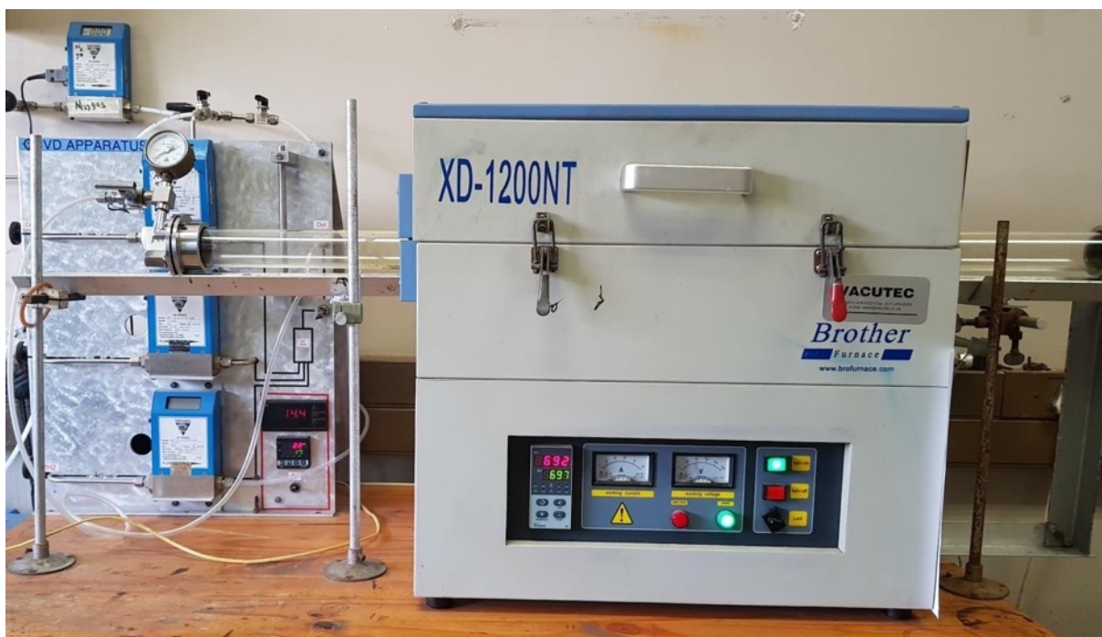
Figure 3.7: The APCVD system used for annealing in this thesis.
