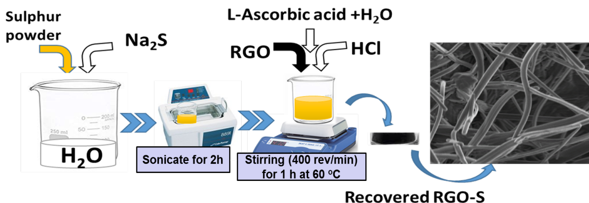
Figure 3.3: Schematic diagram of the synthesis of RGO-S.
