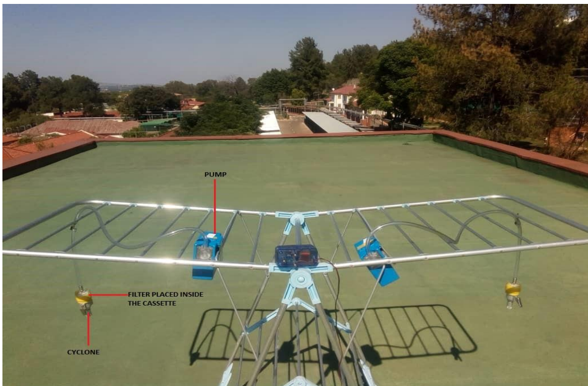
Figure 3.4: Sampling station on top of School of Health Systems and Public and Health building showing the sampling set up.
