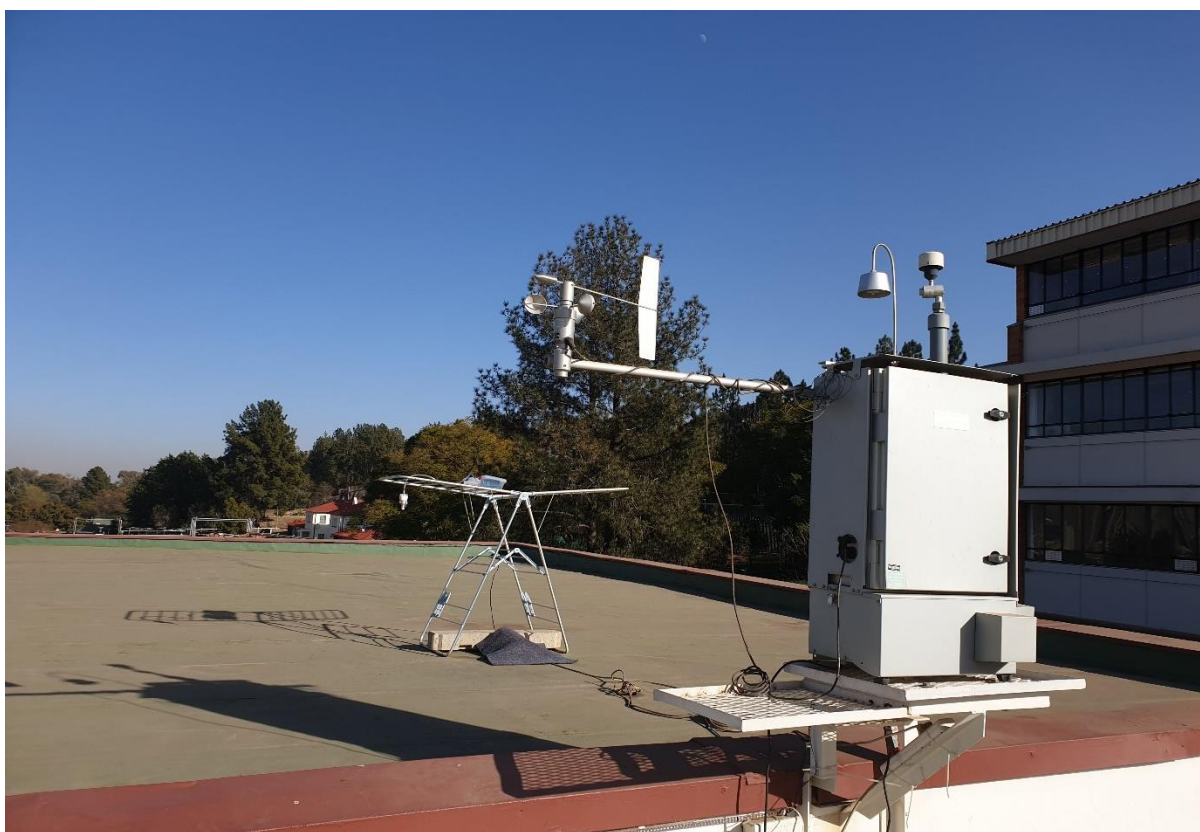
Figure 3.5: Image of Areoqual next to GilAir pump measurements on roof top of School of Health Systems and Public and Health building
