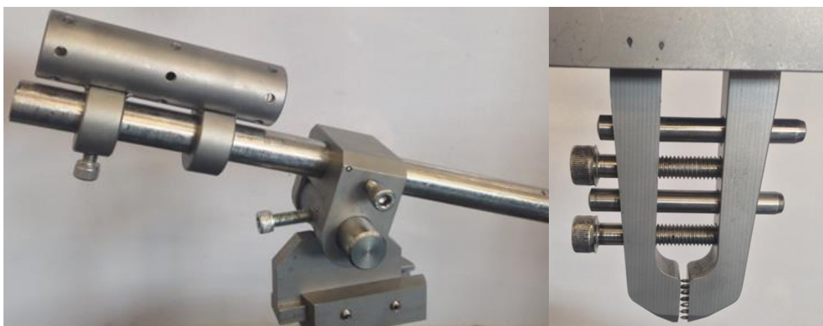
Figure 4.2.1. Clamp on the left designed to hold the humerus around the shaft during testing, holes in clamp allow for screw placement to hold the humerus in place. Clamp on the right designed to hold onto capsular and tendinous strips between the teeth, with added sandpaper to prevent clamp tearing of strips.
