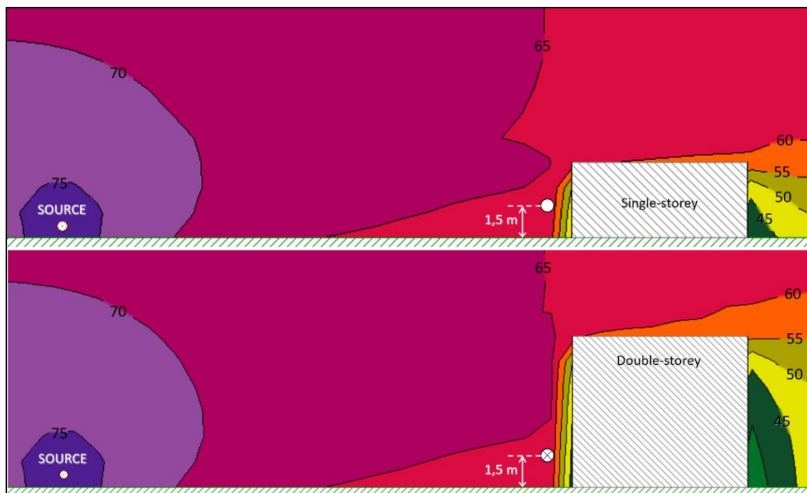
Figure 5-9: Comparison of sound contours in front of single- or double-storey facade for receiver of equal height
