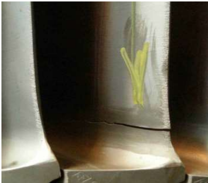
Figure 1-3: Lower aerofoil cracking (Alstom, 2016)
