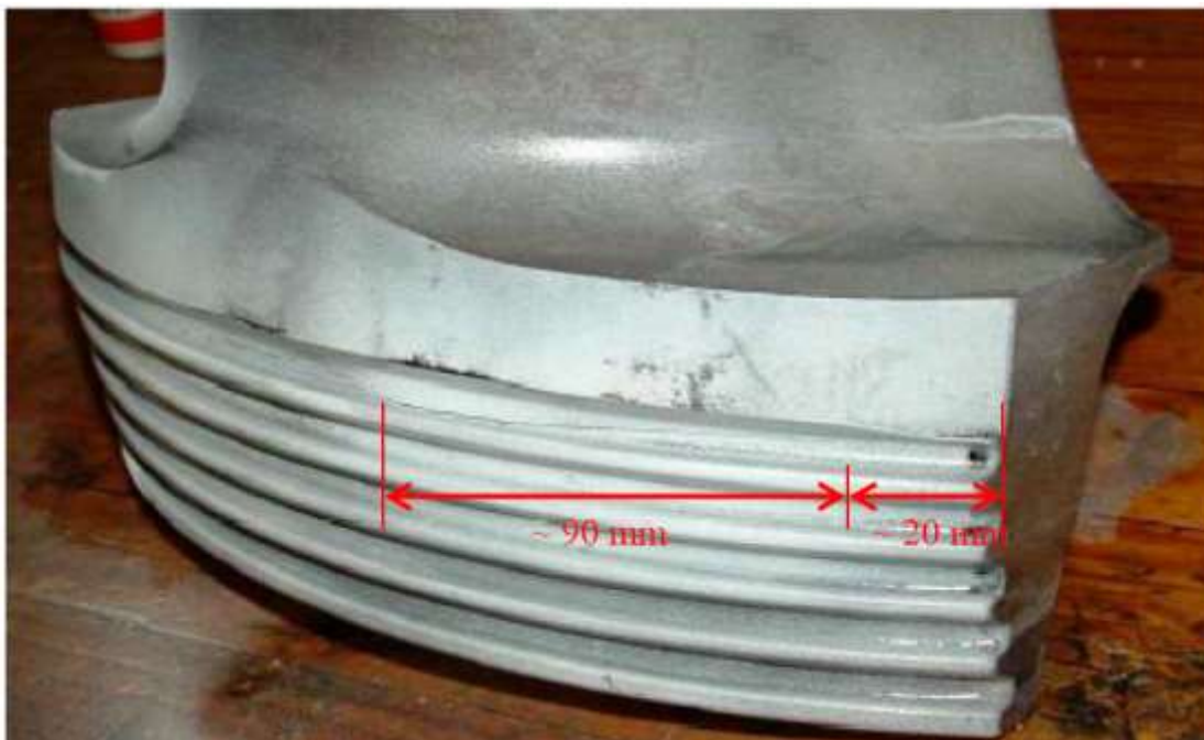
Figure 1-1: Top serration convex cracking
