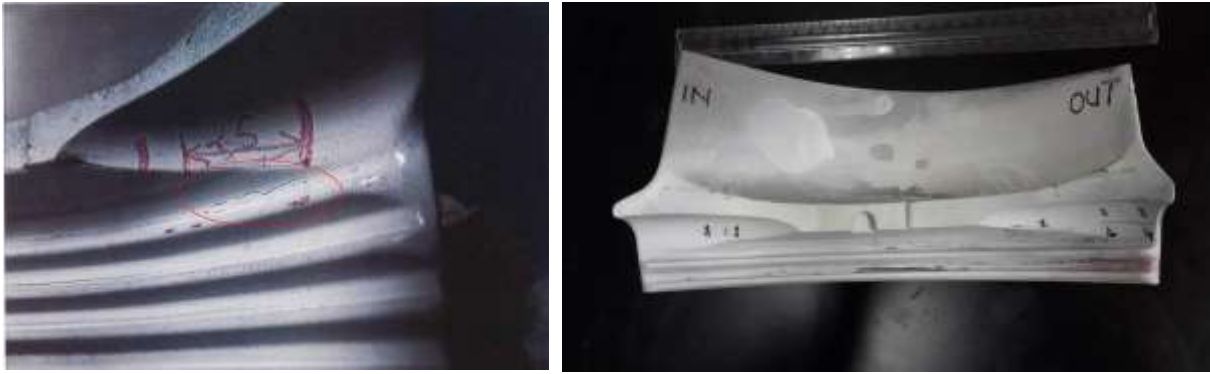
Figure 1-2: Cracks shown on the concave side of the blade
