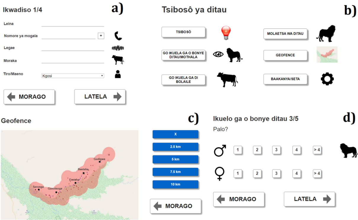
Supplementary Figure 4 – Illustrated draft designs of the lion alert community portal interfaces, showing a) the user registration menu, b) the main menu with core functions: last alert, lion observation report, cattle predation report, lion information, geofence visualization, settings, c) the geofence sub-menu with risk proximities, and d) the lion observation report sub-menu.
