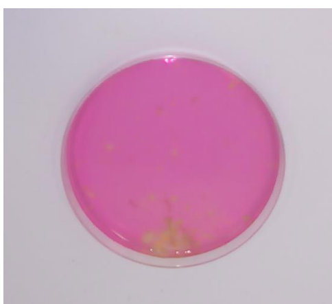
Figure 4.4 Sterilised Co/LCs 10 paste (beige area in lower centre) after 72 hr incubation in DMEM at 37°C.
