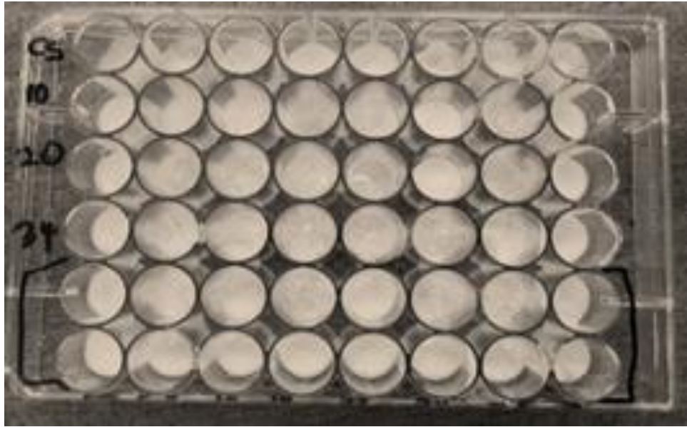
Figure 2.6 Scaffolds prepared in 48-well plates after lyophilisation. The cylindrical scaffolds measured 7 mm in diameter, with a thickness of 4 mm.
