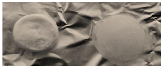
Figure 2.7 Non-neutralised and neutralised scaffolds swollen in PBS pH 7.4. (A) Non-neutralised scaffolds in PBS. From the left showing: chitosan, lauroyl chitosan ( LCs_{10} , LCs_{20} and LCs_{34} ), respectively. Scaffolds before neutralisation were unstable in PBS and fully disintegrated within 4 hr (B) Neutralised chitosan before (left) and 24 hr after (right) saturation in PBS, pH 7.4.
