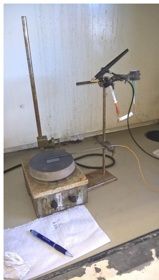
Figure 4.2: The set-up of the spray-pyrolysis system.
