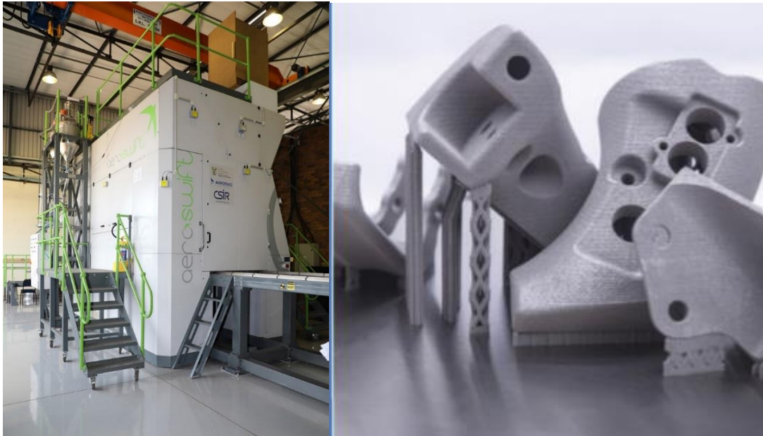
Figure 45. The Aeroswift machine (3D printer) on the left with examples of the parts produced on the right (Source: Vermeulen, 2018).
