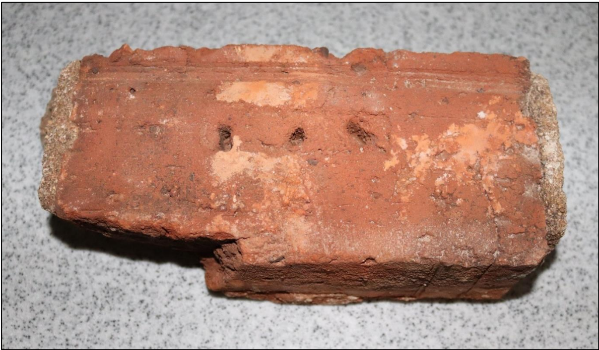
Figure 5.70: Brick from Building 2, indicating the lines and the three prong holes.
