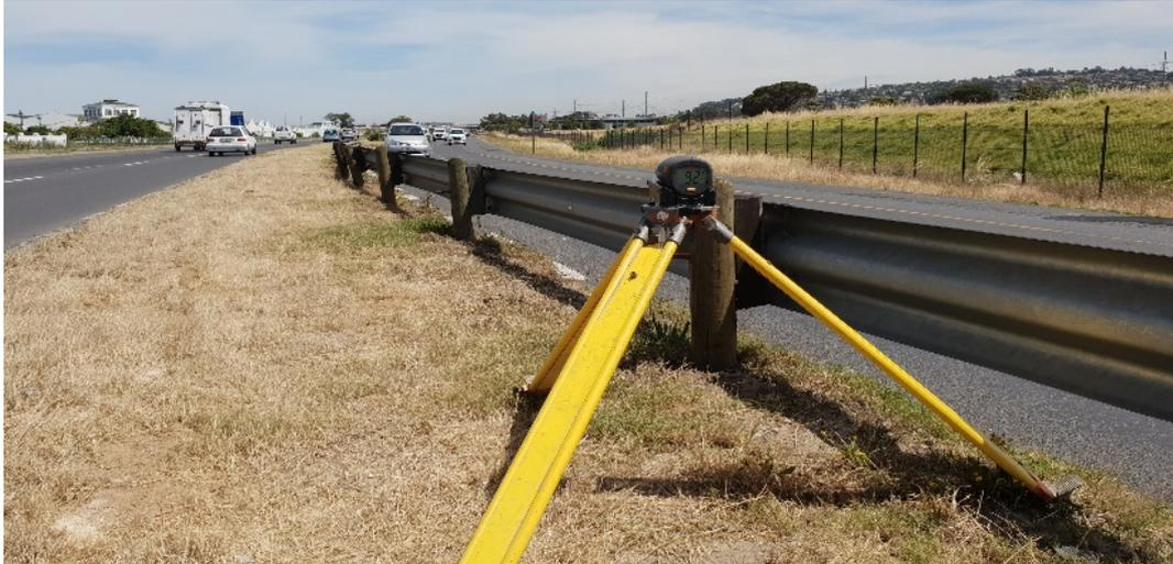
**Figure 3: Radar Gun set up behind Guardrail in the Median**
