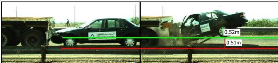
**Figure 7: Bullet vehicle rear wheel elevation**
