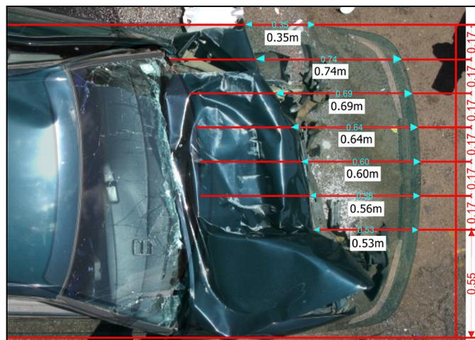
**Figure 11: Bullet vehicle damage measurement**
