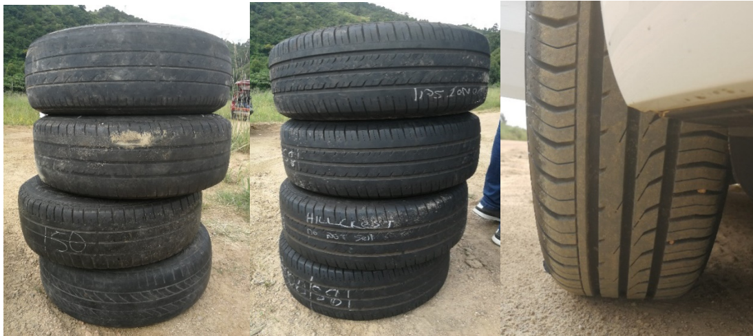
Figure 5: The Smooth (left), 38% tread (middle) and new tyres used for the tests
