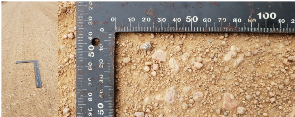
Figure 4: The test road composition of finer aggregate (sand), with some larger aggregate (stone)
