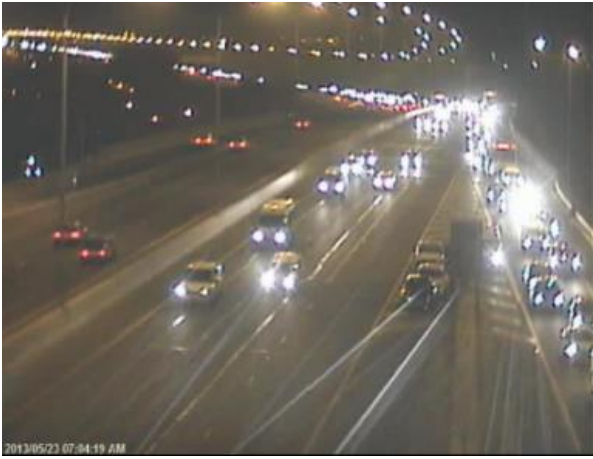
Figure 2: Southbound view along R300 at Strand Road off-ramp illustrating queues spilling back at 07:04 A.M. Source: SANRAL
