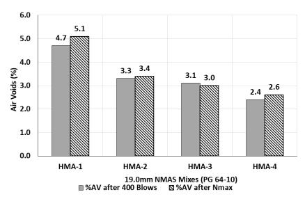
Figure 1: Air void for unmodified PG 64-10 asphalt mixtures after 400 blows Marshall refusal density and Nmax 205 Superpave gyrations
