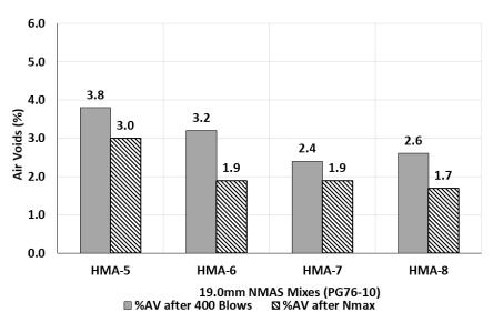
Figure 2: Air void for SBS modified PG76-10 asphalt mixtures after 400 blows Marshall refusal density and Nmax 205 Superpave gyrations
