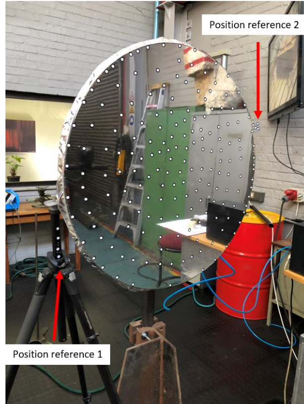
Figure 16: Position marker layout and identification during testing
