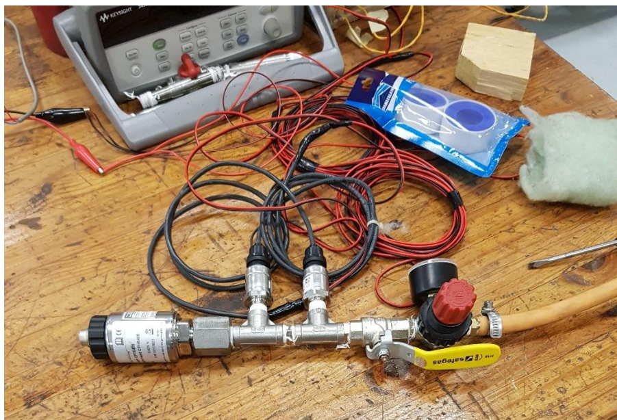
Figure 71: Pressure transmitter calibration setup
