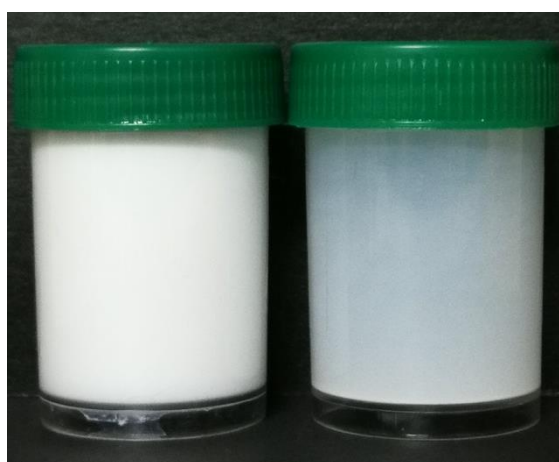
Figure 4.1. Initial appearance of prepared \text{TiO}_2 -water nanofluid samples at 0.25% volume fraction with (left) and without (right) the addition of SDS
