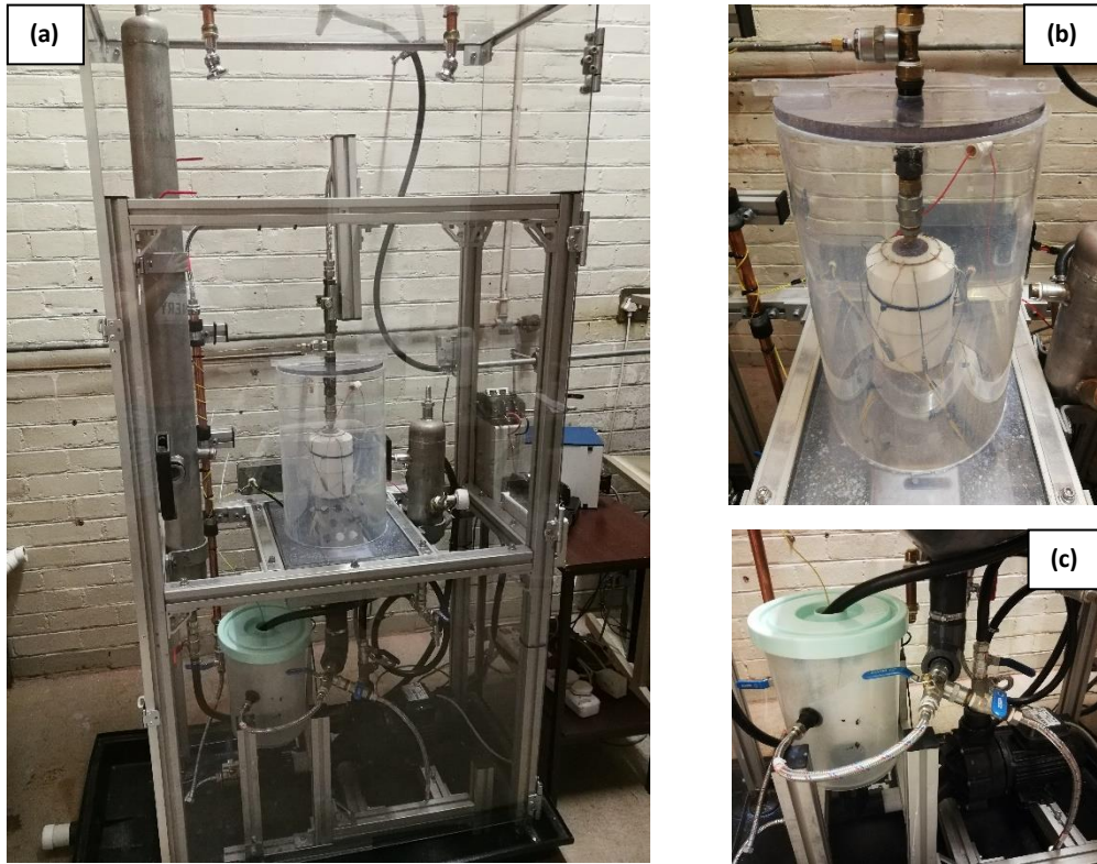
Figure 3.3. Photographic representation of (a) overall jet impingement experimental set-up, (b) close-up of jet and target surface and (c) close-up of main tank and drainage valves
