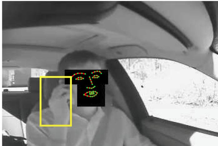
**Figure 2.2.** A cropped region of interest that is extracted to determine the presence of a phone. Taken from [6], © 2015 IEEE.
