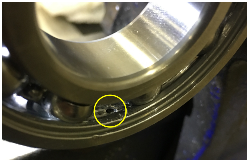
Figure 12: Visible damage on OR after damage level 5.
